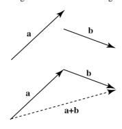
Fig. 3.10 The triangle method of addition
